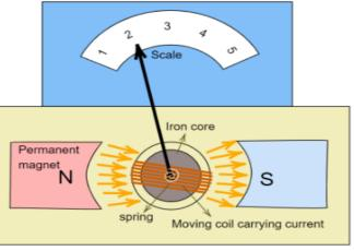
Front view of a Moving Coil Galvanometer
